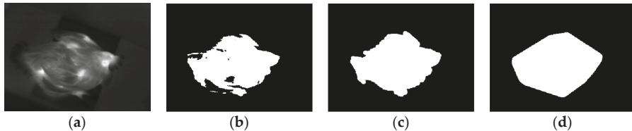
Figure 3. Image pre-processing: (a) Grayscale image; (b) Binary image; (c) Image after morphological processing; (d) Convex hull image.
