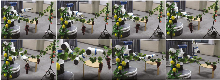
Figure 13. Video frames showing the robot reaching a cluster of plastic grapes, cutting the peduncle, and placing them onto a table.
