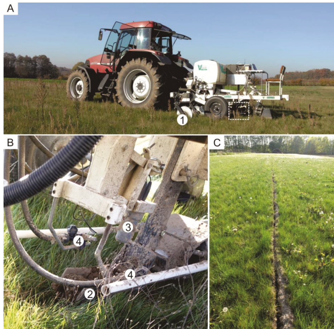
Figure 2. (A) Veris mobile sensor platform, (B) Veris pH-Manager, and (C) furrow cut by the pH sampler trough. Numbers indicate (1) rolling ECA coulter electrodes, (2) pH sampler trough, (3) pH electrodes, and (4) cleaning nozzles.
