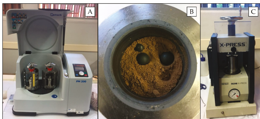
Figure 1. Planetary ball mill (A), loose soil inside the tungsten carbide jars with the tungsten carbide balls (B) and hydraulic press (C), which were used at work.
