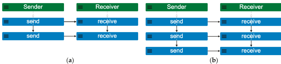
Figure 2. Pre-loaded MP model Example01_simple_message_flow scenarios from (a) scope 2, showing the scenario containing the new maximum of two iterations of send and receive (trace 3); (b) scope 3, showing the scenario containing the new maximum of three iterations of send and receive (trace 4).
