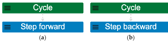
Figure 3. Initial event trace outputs of the Cycle_ISP_v1 model, run for scope 1: (a) Cycle steps forward; (b) Cycle steps backward. Neither scenario contains any repetition and therefore only represents part of a cycle’s behavior.
