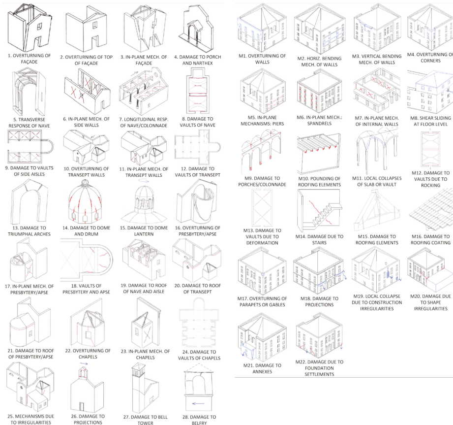
Figure 3. Example of mechanisms for masonry churches and buildings adopted in DataBAES forms, as shown in church (A-DC, 28 mechanisms) [19] and palace (B-DP, 22 mechanisms) [20] survey forms.
