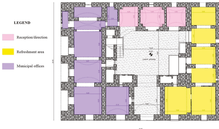
Figure A10. Offices' ground floor plan.
