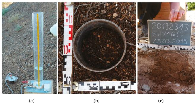
**Figure 4.** (a) Single-ring infiltrometer; (b) plot record before the experiment; (c) profile of the infiltration plot after experiment.
