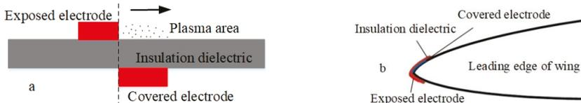
Figure 7. Surface dielectric barrier discharge actuator. (a): structure; (b): position layout.
