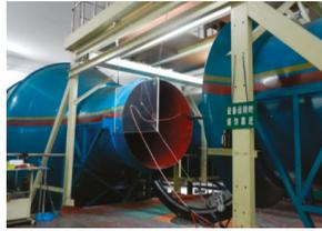
Figure 1. FL-5 wind tunnel open test section.
