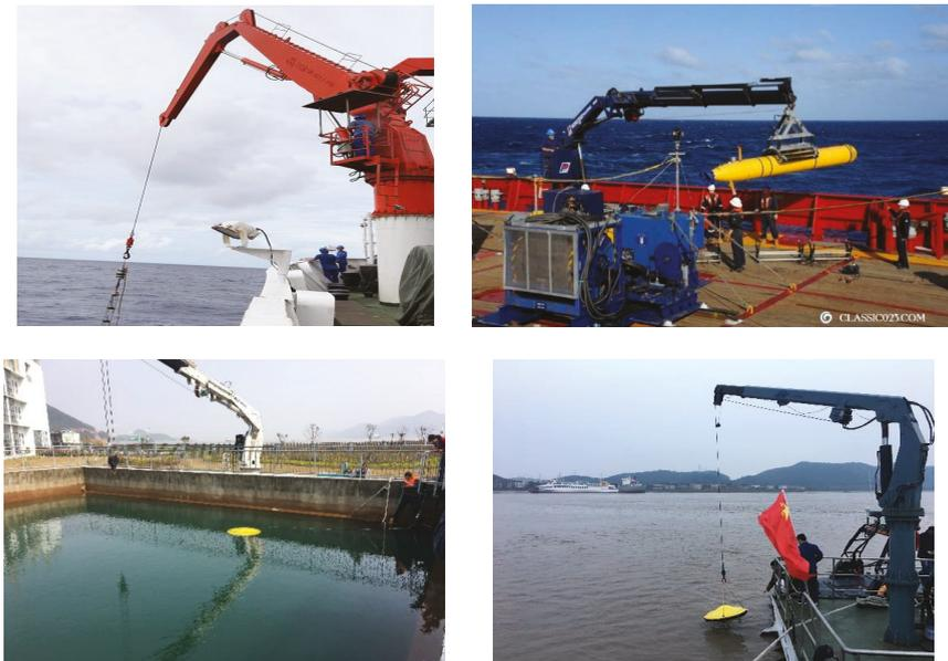
**Figure 2.** Conventional launching and recovery system of a single-arm crane.
