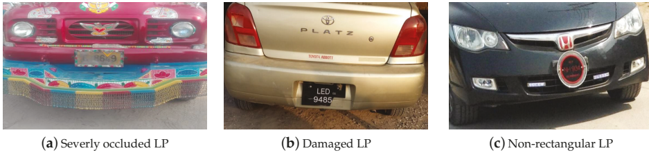
Figure 10. Vehicle images where LPs are not correctly segmented due to various reasons.
