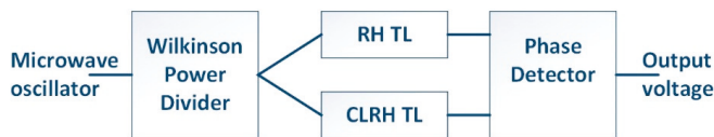
Figure 2. Block diagram the proposed microfluidic CLRH sensor (RH LT–right handed transmission line, CLRH TL–composite left-right handed transmission line).
