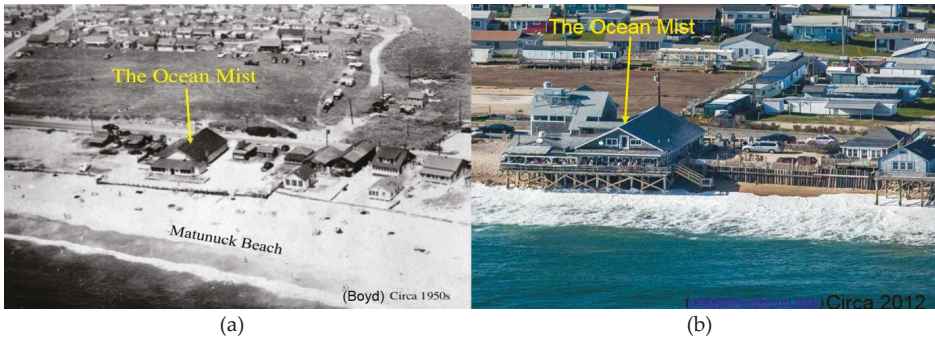
Figure 3. Photographs of a local restaurant in the study area from: (a) the 1950s; and (b) 2012, showing the loss of shoreline due to erosion [2].
