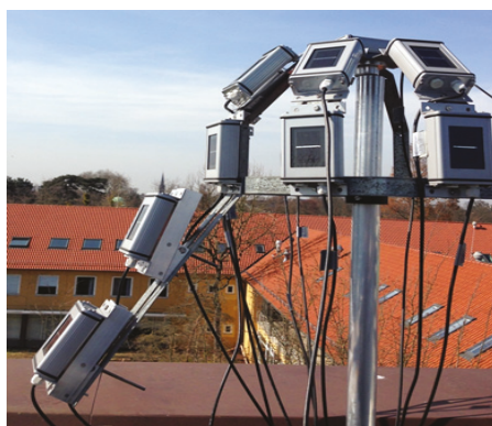
Figure 1. Set of solar PV devices based on silicon sensors mounted in several different tilt angles and orientations, operational at the IMUK (Institute for Meteorology and Climatology) [IMUK, 2017].
