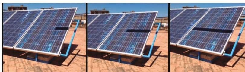
Figure 8. Shaded panel case 1, 2 and 3. In case 1 shadow can vary from 225 to 450 cm 2 ; which corresponds to one interruption of a line of cells; in case 2 shadow varies from 450 to 900 cm 2 , which corresponds to two interruption of lines; case 3 corresponds to the interruption of the panel.
