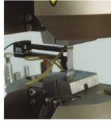
Figure 7. Experimental setup of a uniaxial tension test.
