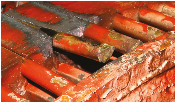
Figure 2. Damaged rotor cage—visible sheared bars of the starting cage.
