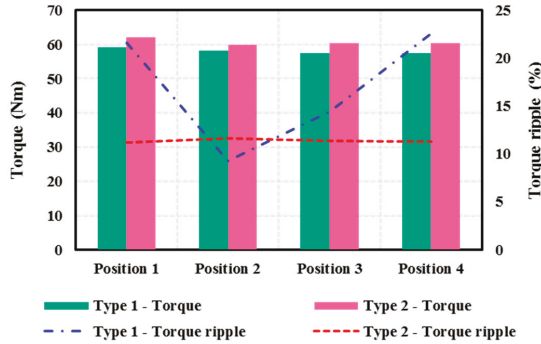
Figure 8. Torque production for each PM position.
