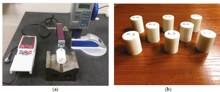
Figure 2. (a) Surface roughness measurement setup (b) Printed samples for experiment 1.
