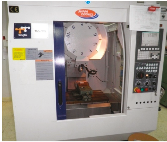
Figure 4. Tongtai TMV510 machining center equipped with a Fanuc Control Numeric Computer (CNC).
