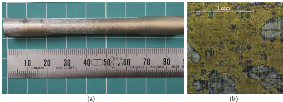
Figure 9. (a) General image of corroded specimen ( V_c = 60 m/min, f = 0.2 mm/r). (b) Detail ( \times 72 ) of the corroded surface.
