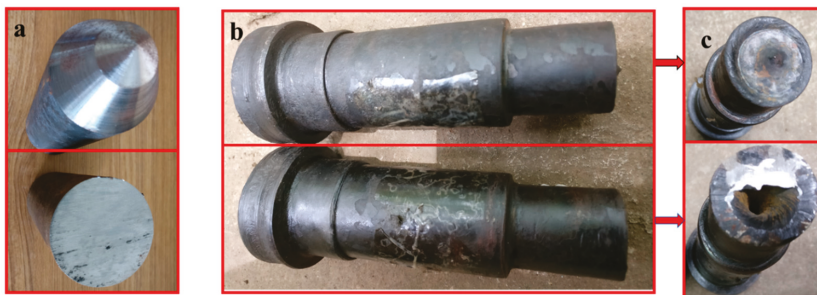
Figure 16. Billets and rolled products: (a) comparison of billets; (b) lateral comparison of rolled products; (c) axial comparison of rolled products.
