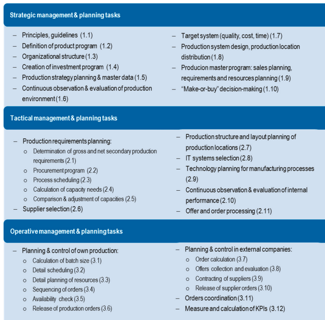
Figure 4. Production management and planning tasks acc. to time horizons (own elaboration).
