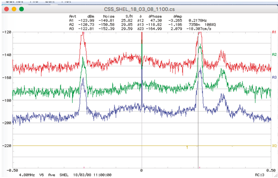
Figure 1. An example of an uncontaminated radar spectrum obtained from a SeaSonde system, measured at Shelter Cove, California, 8 March, 2018, 11a.m. range 18 km. Radar-echo spectral power (dB) from the three SeaSonde antennas is plotted vs. Doppler frequency for the Loop 1 antenna (A1, red), the Loop 2 antenna (A2, green) and the monopole (A3, blue). The curves are offset by 20 dB for better visibility. The first-order Bragg peaks at Doppler \pm 0.22 Hz are surrounded by second-order echo, with the second-order peak especially visible to the right of the positive Bragg peak. The yellow line is an indicator of spectral quality.
