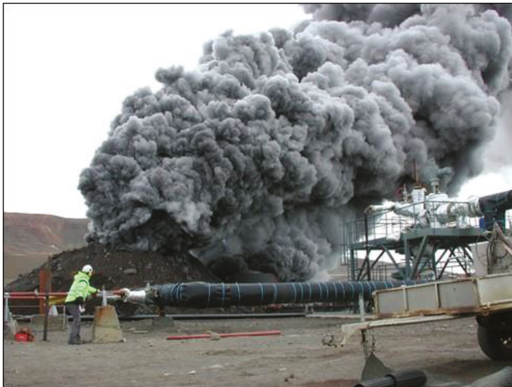
Figure 17. The beginning of a flow test of IDDP-1 (photo G. Ó. Friðleifsson).
