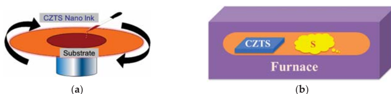
Figure 2. Fabrication process of CZTS films: (a) fabrication of CZTS precursor by spin-coating and (b) the sulfur vapor annealing process.
