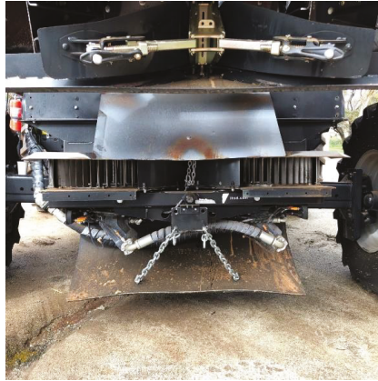
Figure 2. Mechanical seed destruction unit (iHSD) mounted in a commercial combine harvester.
