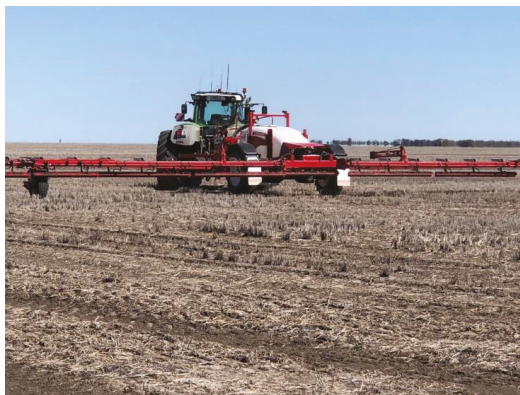
Figure 3. Autonomous site-specific weed control with a real-time weed detection and application sprayer in a fallow field.
