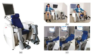
**Figure 1.** The prototype of the LLR-Ro: (a) The prototype of the LLR-Ro; (b) The movable seat separated from and grouped into the LLR-Ro; (c) The back angle of the movable seat altered from 110° to 170°.
