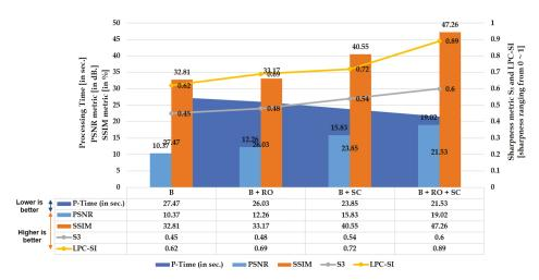
Figure 4. Quantitative: Significance of proposed cumulative set aggregation loss and refinement scheme with respect to image quality, edge stretching, and processing time on distorted KITTI dataset.
