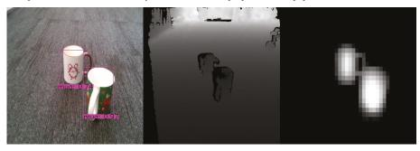
Figure 13. An example of real world object classification using the proposed network model: segmented and classified RGB frame (left), depth frame (middle), and predicted depth mask (right).
