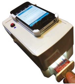
Figure 4. Light box with embedded electronic lighting system, which minimizes the relative movement between the smartphone and the test and the effects of external illumination changes.
