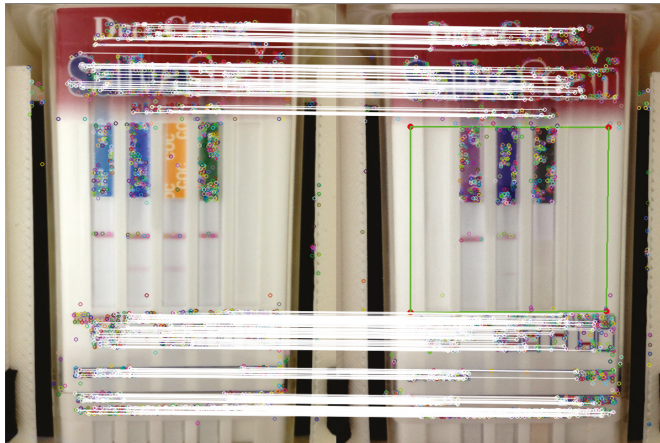
Figure 5. Matching process between oriented FAST and rotated BRIEF (ORB) descriptors in the template image (left) and original image (right). White lines denote the matched points. In green is depicted the searched region of interest that contains the strips in the actual processed image.
