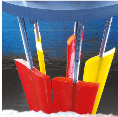
Figure 23. 3D printed blades installed on the prototype.
