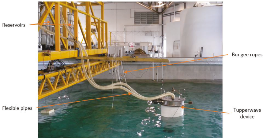
Figure 5. Physical model of the Tupperwave device.
