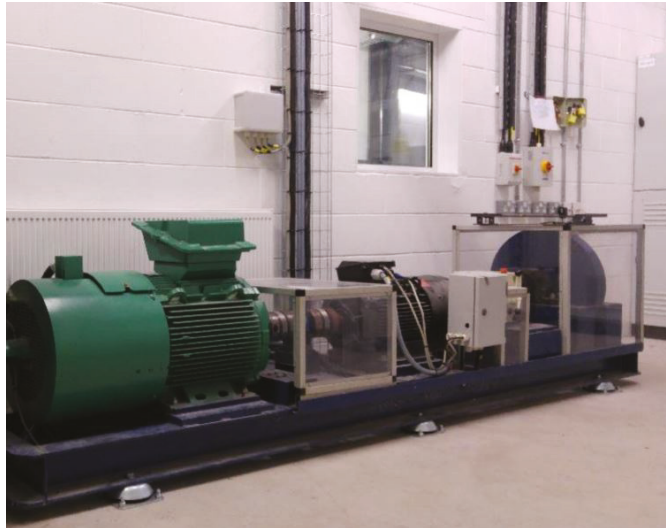
Figure 13. Rotary test rig of the Lir National Ocean Test Facilities (Lir-NOTF), used to emulate the turbine-generator systems of the devices.
