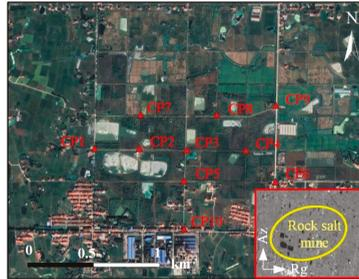
**Figure 12.** Locations of the benchmarks in the rock salt mine (the corresponding amplitude images are shown in the red rectangle in the southeast corner).
