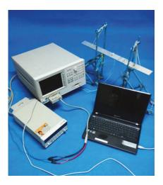
Figure 3. Experimental setup for impedance measurements on the bolt-jointed aluminium beam.
