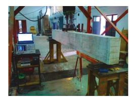
Figure 19. Experimental setup for the reinforced concrete beam externally strengthened with an FRP strip.
