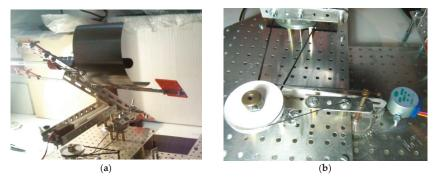
Figure 4. Details of the two axis tracking mechanism. (a) Linear actuator; (b) Stepper motor.
