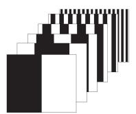
Figure 8. Structured light typical patterns.
