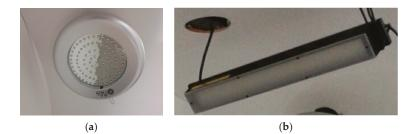
Figure 2. Illumination subsystem (a) Daytime LED panel; (b) Nightime LED panel.
