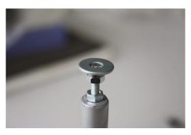
Figure 6. Detail of the washer-ball bearing assembly supported by the nut, without the arm.
