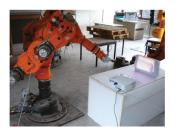
Figure 16. Robot positioning using structured light [96].
