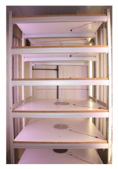
Figure 8. Rack composed of 5 flight mills.
