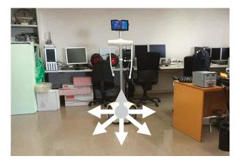
Figure 3. Representation of the direct motion capabilities of the APR.
