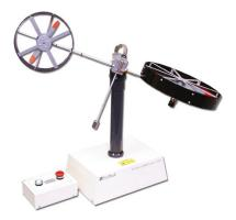
Figure 1. Twin rotor MIMO system (TRMS).
