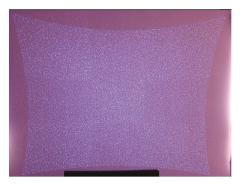
Figure 10. Projected pattern in Light coding.
