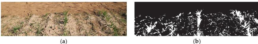
**Figure 13.** (a) Image acquired by the robot of the end of a crop row. (b) Segmented image of Figure 13a. The number of pixels that is associated with vegetation (white pixels) is less than 80% of the number of pixels in the reference image (Figure 6), and the robot location is very close to the output point that is defined in the plan for the row that is being scouted. Thus, the robot determines that it has reached the end of the crop row.
