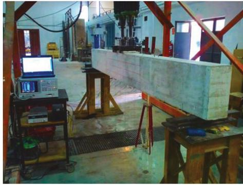
**Figure 19.** Experimental setup for the reinforced concrete beam externally strengthened with an FRP strip.
