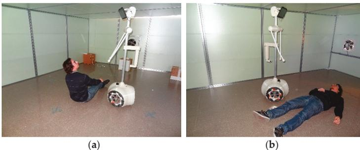
**Figure 18.** Simulation of the APR used as a fall detector (a) with activity and (b) without activity.
