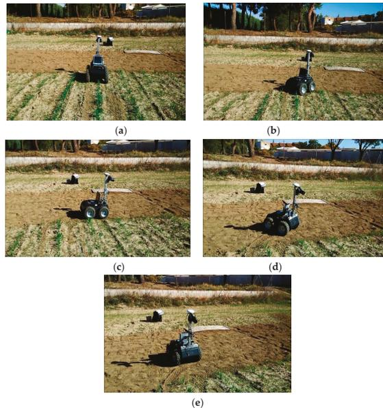
**Figure 19.** Sequence of manoeuvres performed by the robot to change rows. (a) corresponds with manoeuvre 1 in Figure 14, *i.e.*, the straight-line forward movement; (b) with the circular-arc movement, manoeuvre 2; (c) with straight-line forward movement, manoeuvre 3; (d) with reverse circular-arc movement, manoeuvre 4; (e) with straight-line forward movement, manoeuvre 5. Video can be found in [65].
