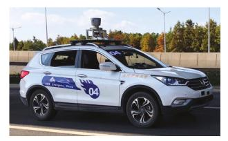
**Figure 6.** Our experimental platform. It is equipped with a Velodyne HDL-64E Lidar, a Xsens MTI300 IMU, two photoelectric encoders, a NovAtel SPAN-CPT GNSS/INS system, and a Nova 5100 industrial computer.
