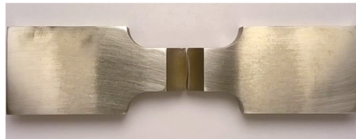
(b) With LSP, PD = 900 cm 2 , SD = 2.5 mm, crack in the middle of the specimen
