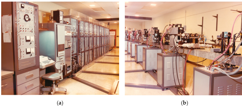
Figure 1. The Battelle Compagnie Générale Electrique (CGE) VD-640 Q-switched laser became operational in 1970 and was used for laser shock investigations to the mid-1990s: (a) capacitor banks; (b) laser rod amplifiers.
