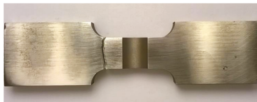
(c) With LSP, PD = 1600 cm 2 , SD = 2.0 mm, crack at the edge of LSP area
