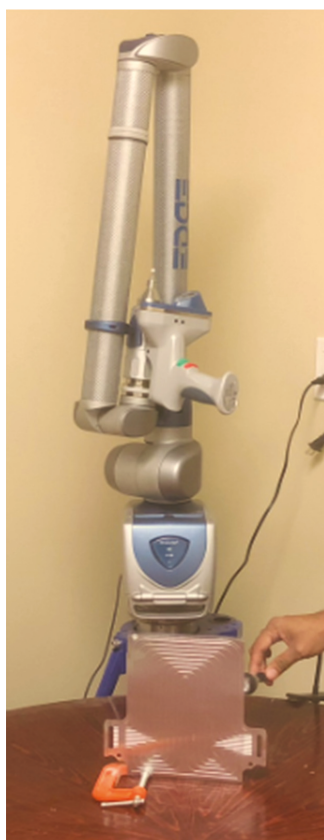
Figure 2. Laser scanning set-up.
