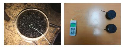
Figure 1. Thermo-sensor inside the specimens.
