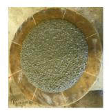
Figure 6. Flow table test.
