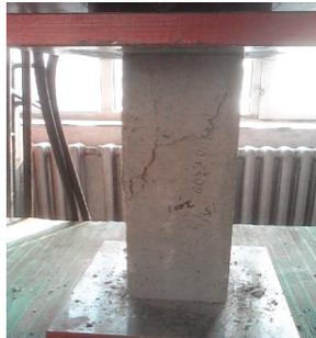
Figure 7. Cube for material test.
