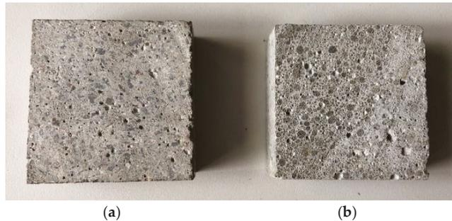
**Figure 8.** Cross-section of (a) the control sample (CS) and (b) E100 mixtures samples with uniform distribution of EGA in the cement matrix.
