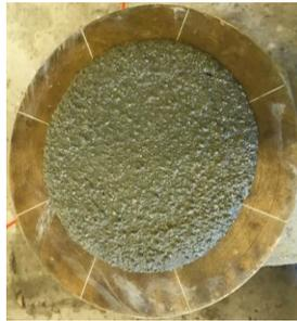
Figure 6. Flow table test.
