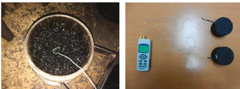
**Figure 1.** Thermo-sensor inside the specimens.
