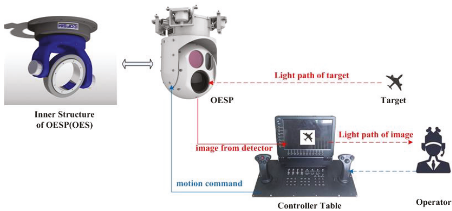
Figure 1. Principle of the opto-electric servo platform (OESP).
