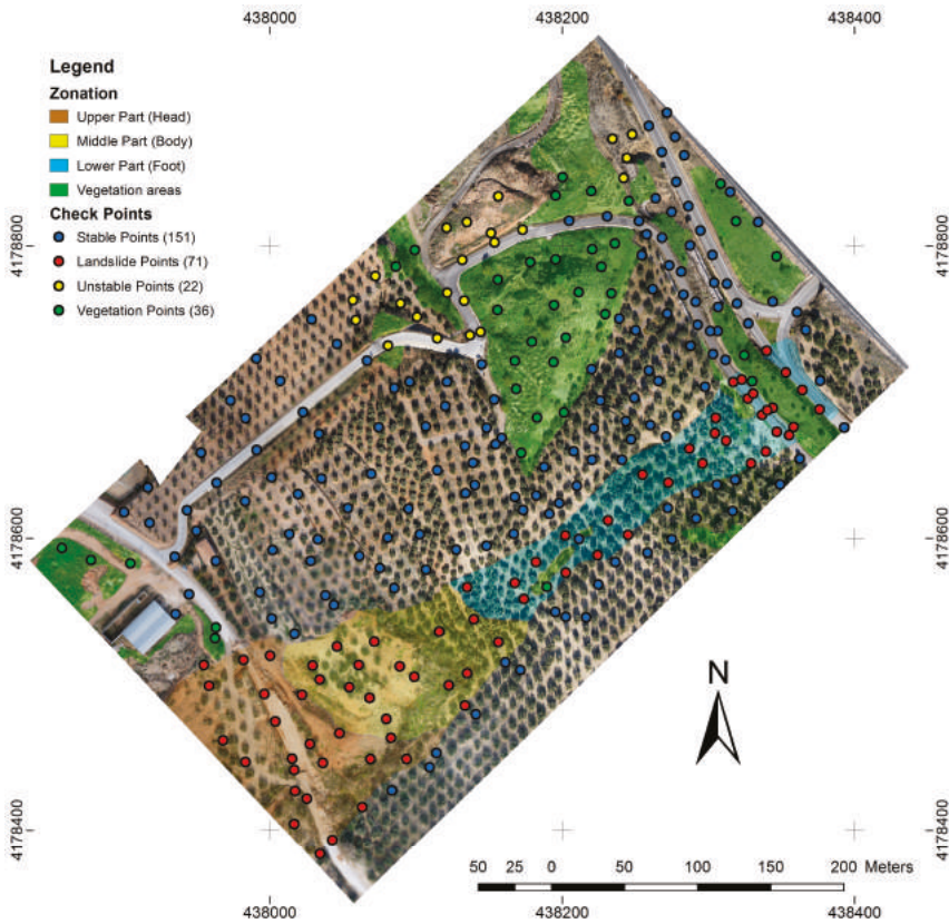
Figure 8. Distribution of DSM check points in the study area. Coordinates are in ETRS89, UTM-30.
