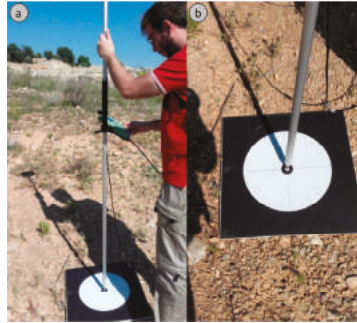
Figure 6. (a) GCP targets and their measurement by DGNSS; (b) Detail of the targets.
