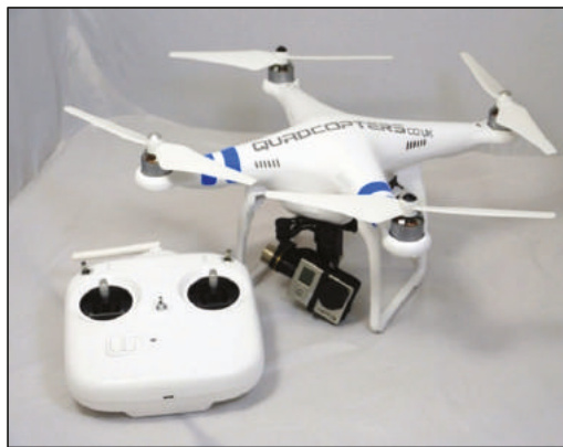
Figure 6. The DJI Phantom 2 unmanned aerial vehicles (UAV) drone equipped with the GoPro camera used in this study.
