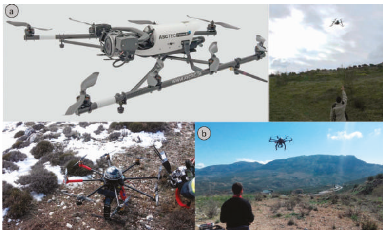
Figure 4. UAV equipment used in this study: (a) AscTec Falcon 8; (b) ATyges FV-8 Drone.
