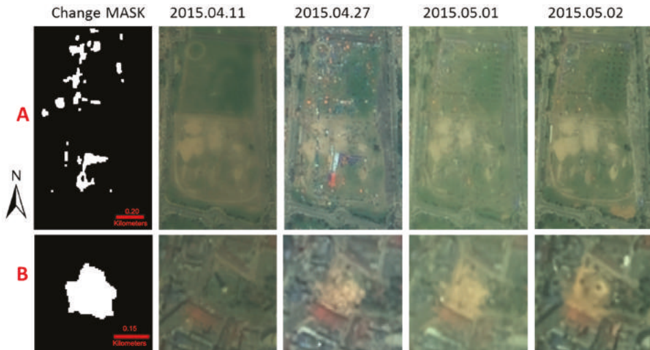
Figure 27. The temporal change detail map of two scenes ( A shows a series of changes in Center Park from 27 April to 2 May and B shows the change of a collapsed tower).
