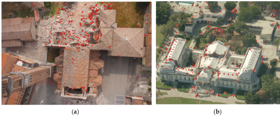
Figure 9. Detected SURF points are plotted on the image. (a) Strongest 300 SURF points among 4032 \times 3024 pixels; (b) strongest 300 SURF points among 977 \times 835 pixels. Images © Pictometry.
