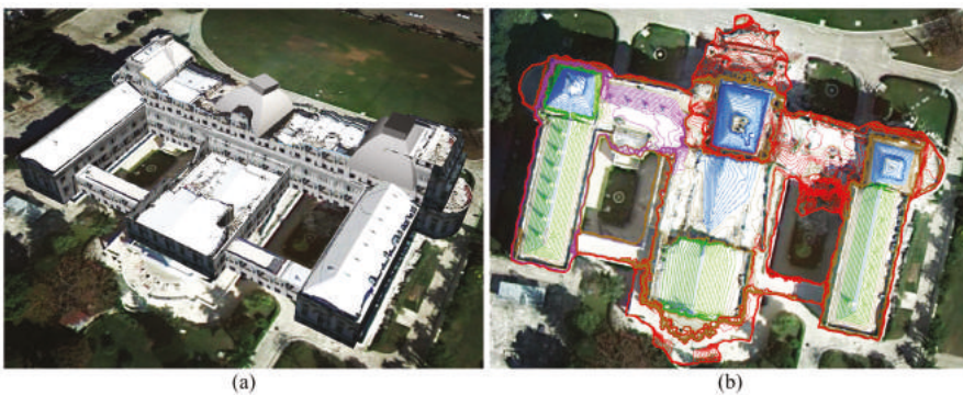
Figure 5. The spatial patterns of complex roof surfaces are represented by contour clusters: (a) The complex surface of Haiti’s National Palace, which was destroyed in the 2010 Haiti earthquake (obtained from Google Earth); (b) Contour clusters of the roof are rendered in different colors according to different surface or structural morphologies, such as contours of surfaces with debris (red), twisted surfaces (purple) and inclined roof structures (blue), which are jagged or irregular, and contours of intact surfaces and structures (green) are compact and regular.
