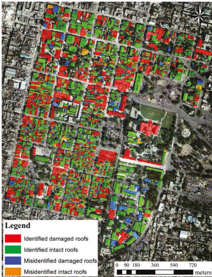
Figure 10. The validated results of damaged roof detection, where correctly detected intact roofs (identified intact roofs) are colored green, correctly detected damaged roofs (identified damaged roofs) are colored red, undetected damaged roofs (misidentified intact roofs) are colored yellow, and undetected intact roofs (misidentified damaged roofs) are colored blue.
