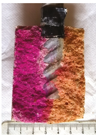
Figure 2. Image of a broken reinforced sample previously exposed to \text{CO}_2 , after the use of phenolphthalein (left) and yellow alizarin (right) indicators to check pH.
