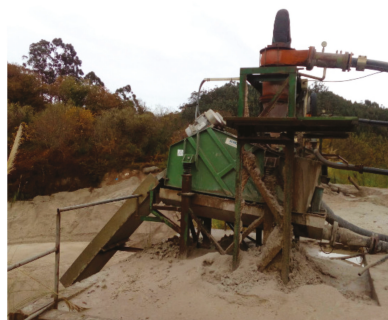
(b) Waste draining system
