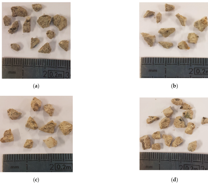
Figure 2. Samples of new pastes before MIP tests (a) NP0, (b) NP30, (c) NP50 and (d) NP100.
