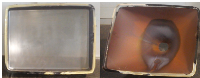
Figure 1. Left, front part cathode ray tube (CRT F ); right, rear part (CRT R ).
