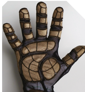
Figure 8. Tactile-sensing glove composed from various sensing patches sewed onto a very thin and breathable base glove. Individual sensing patches are further subdivided into taxels by etching away the conductive silver coating. The corresponding insulating gaps are clearly visible as dark lines in contrast to the bright taxels regions.
