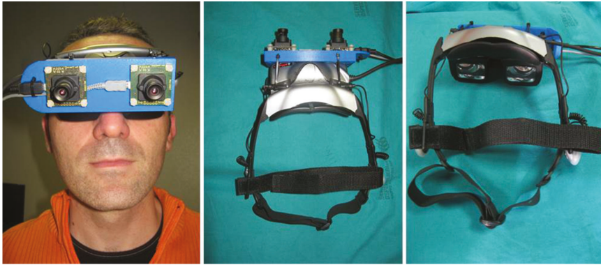
Figure 2. Video see-through head-mounted display (HMD) obtained by mounting two external cameras on top of a commercial 3D visor.
