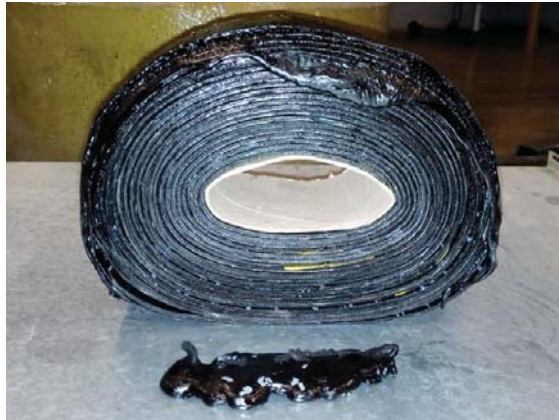
Figure 18. Heated asphalt roll after 8 min of heating.
