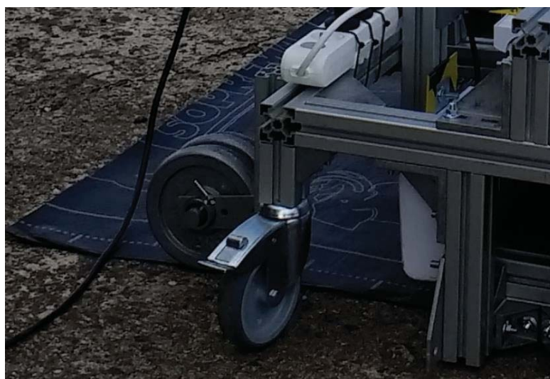
Figure 11. Detail of the small drum roller for the sealing of overlaps.
