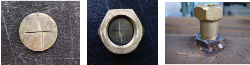
Figure 2. Pipeline defect model and method for fixing it.
