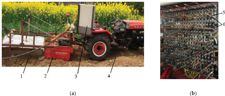
Figure 1. Custom-made soil steam disinfection (SSD) machine: (a) SSD machine; (b) steam disinfection pipe layout. 1. Steam disinfection mechanism. 2. Rotary tiller. 3. Control box. 4. Tractor. 5. Steam pipe. 6. Steam pipe spacing (SPS).
