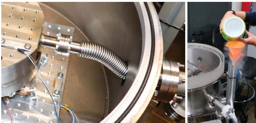
Figure 17. Connection to the internal LN 2 supply through a flexible bellow (left). Connection to the external LN 2 supply by direct pouring (right).
