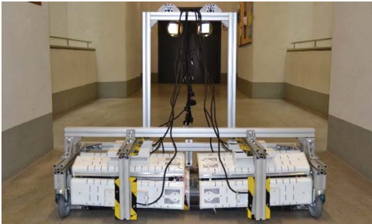
Figure 12. Prototype of the equipment for the fast installation of asphalt roofing based on infrared heaters.
