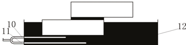
Figure 6. Test shear sample placed in the water bath.
