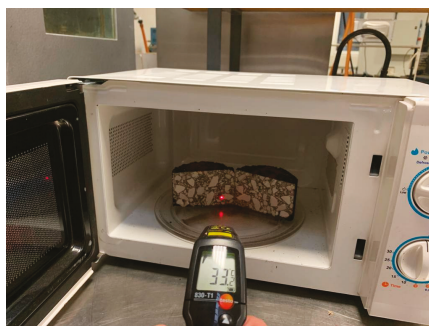
Figure 4. Internal temperature measurement.
