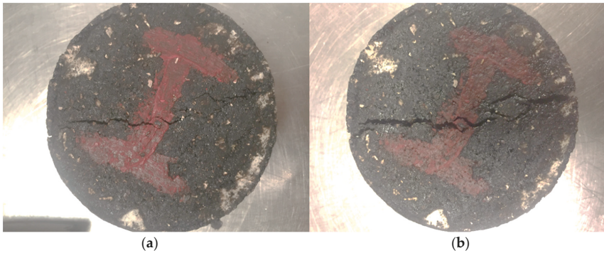
Figure 7. The broken specimen before heating (a), and the enlargement of the crack after the heating without rubber bands (b).
