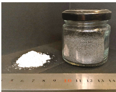
Figure 1. Mass of 2.50 g of limestone filler under 0.063 mm (left) and graphene nanoplatelets (right).
