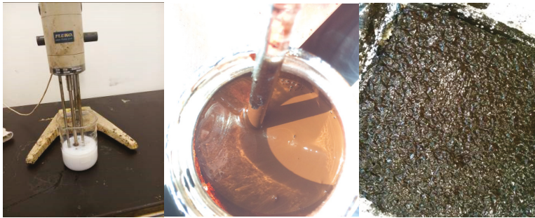
Figure 1. Preparation process of nano TiO 2 epoxy emulsified asphalt and mixtures.
