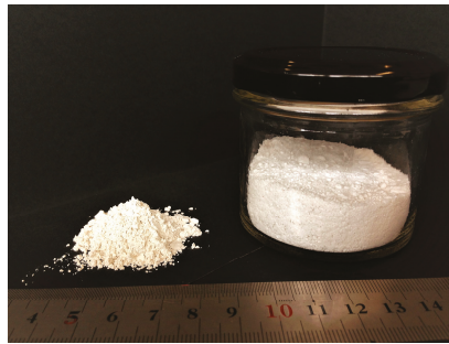
Figure 1. Mass of 2.50 g of limestone filler under 0.063 mm (left) and nanosilica (right).
