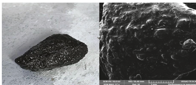
Figure 16. A piece of aggregate coated with Graphene Nano-Platelet (GNP)-modified binder.
