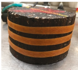
Figure 6. Simulation of in situ confining conditions of the asphalt pavements.
