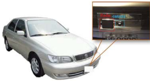
Figure 11. Experimental car and sensors setup.
