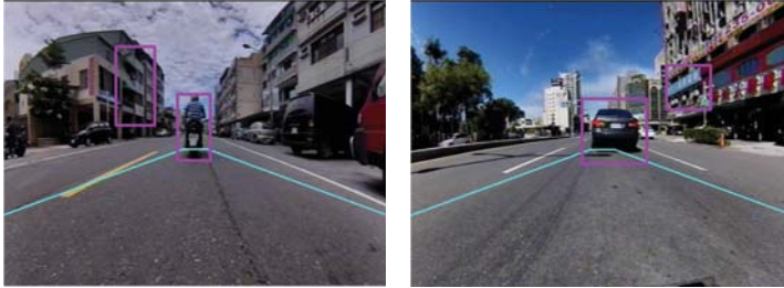
Figure 17. Error detection of the Haar-like algorithm.
