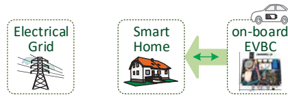
Figure 11. On-board EVBC: Vehicle-to-home (V2H) operation mode (as an off-line uninterruptible power supply).
