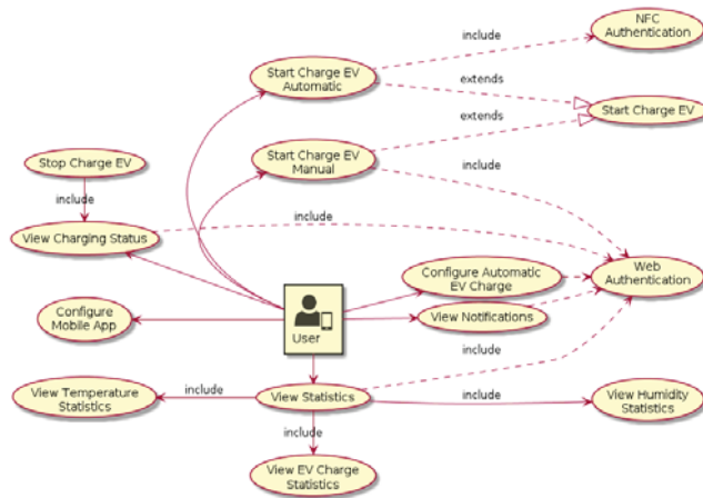
Figure 5. Use case diagram of the developed mobile app.
