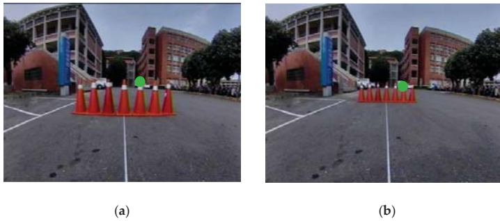
Figure 10. Diagram of same image coordinates correspond to different radar coordinates (a) Radar detection distance is 2.2 m and (b) Radar detection distance is 4 m.
