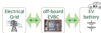
Figure 14. Integration of an off-board EVBC into the electrical power grid for G2V and V2G operation modes.
