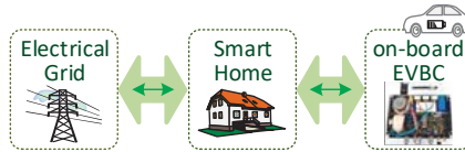
Figure 7. On-board EVBC: vehicle-to-grid (V2G) operation mode.
