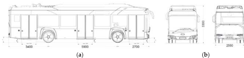
Figure 2. Overall dimensions of the Solaris 12 E bus. (a) side view (b) front view.
