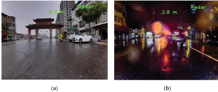
Figure 16. Detection results of radar subsystem for a rainy day, (a) motorcycle and (b) car.
