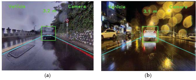
Figure 19. Detection results by vision-based subsystem for a rainy day, (a) daytime and (b) nighttime.
