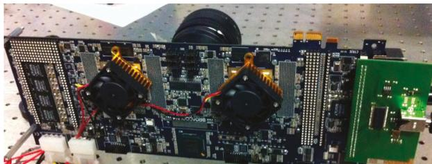
**Figure 15.** Physical appearance of the camera based on SwissSPAD; a daughterboard hosting the chip is electrically connected to a motherboard hosting two Xilinx-IV that process the raw frames generated by the chip and format them to send them through a USB2 link.
