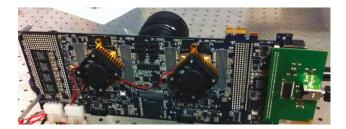
**Figure 15.** Physical appearance of the camera based on SwissSPAD; a daughterboard hosting the chip is electrically connected to a motherboard hosting two Xilinx-IV that process the raw frames generated by the chip and format them to send them through a USB2 link.
