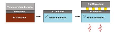
Figure 3. Transfer and bump bonding.
