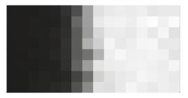
**Figure 8.** Image taken with a PAPD test array biased at -32 V back bias with left part of the array covered at roughly half full-well capacity.
