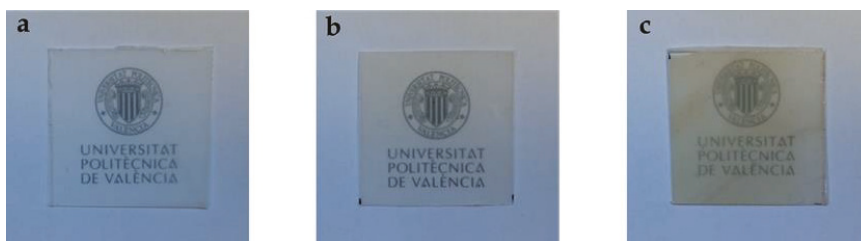
Figure 1. Visual appearance of the bio-based high-density polyethylene (bio-HDPE) films containing different amounts of gallic acid (GA): (a) Bio-HDPE; (b) Bio-HDPE + 0.3GA; (c) Bio-HDPE + 0.8GA.
