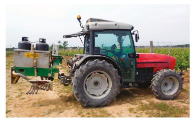
**Figure 2.** The flaming machine PFV-600 (Officine Mingozzi, Ferrara, Italy) coupled with a SAME Frutteto 100 (SAME, Treviglio, Italy) tractor.
