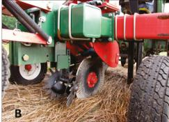
Figure 4. (A) RJ Equipment $^{\circledR}$  no-till transplanter, with the additional custom designed sub-frame to accommodate a custom subsoiler shank (subsoiler used is pointed by arrow) for a single combined subsoiling and transplanting operation. (B) Row cleaners were mounted for cover crop residue management.
