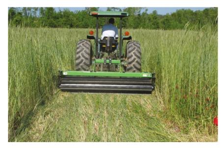
**Figure 2.** Cereal rye crimson clover mixture being rolled/crimped by an experimental patented 1.8 m wide 2-stage roller/crimper.
