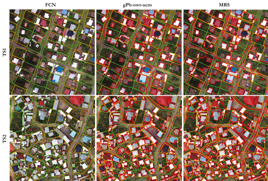
Figure 6. The error map of the investigated techniques. Yellow lines are TP; red lines are FP; and green lines are FN.
