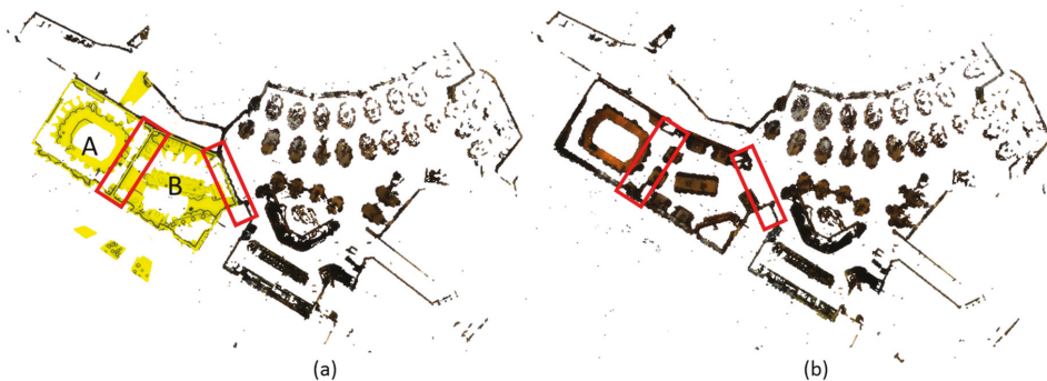
Figure 13. The figure shows the top view of two epochs of our use case. The floor and ceiling are removed for a clear visualization. (a) The data is collected by a Riegl terrestrial laser scanners (TLS) [45] (rooms A and B in yellow) and is co-registered with the data collected by the Viametris system [56]. (b) The second epoch is also collected by the Viametris system and the walls in the red rectangles are removed.
