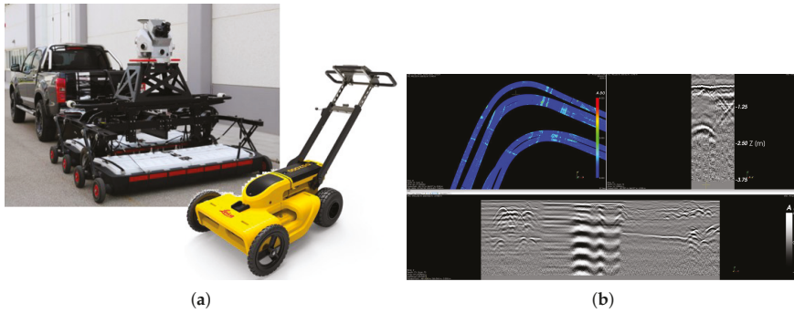
Figure 4. Examples of GPR instruments (a) and GPR data (b); the data show a radargram of a longitudinal cross section of the top-most about 2.85 m along an asphalt paved road (bottom), a perpendicular cross section of one lane (top right) and the top view of the scanning tracks covered by GPR measurements (top left).
