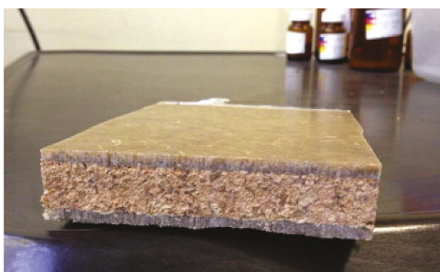
Figure 26. Eco-sandwich with core in granulated cork and skins in hemp/bio-resin. Reprinted from [101], © 2020 with permission from Elsevier.
