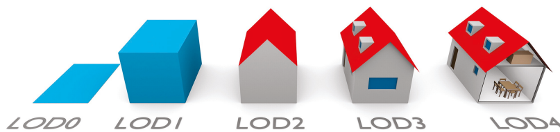
Figure 2. Visualization of LOD0 to LOD4 in the CityGML format [31].
