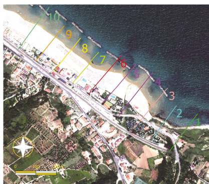
Figure 8. Ten transects every 100 m, drawn from the land to the sea, to calculate the intersection between them and seven shorelines extracted from WorldView-2, WVWI, J-Net Dynamic on the VHR image, Sentinel-1, Sentinel-2, Canny and J-Net Dynamic on the HR image.
