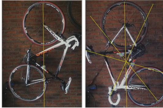
**Figure 2.** Determining the center of mass of a bicycle: orthogonal lines are the most accurate.
