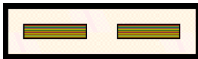
Figure 21. Design I: forward-type transformer for m = 215 : planar E-core and 200 \mu\text{m} copper foil.
