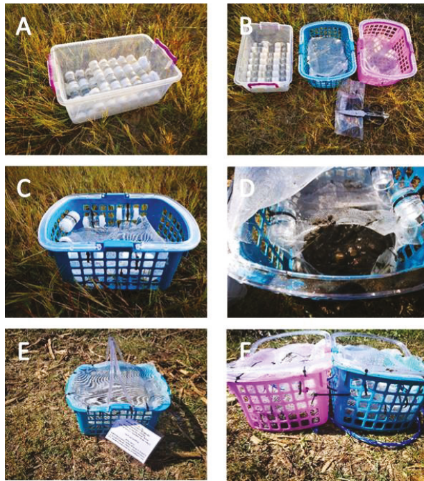
Figure 3. Steps taken to assemble the plastic baskets for the artificial mussels and transplanted clams. (A) Storage of artificial mussels before deployment. (B) Plastic baskets in which the artificial mussels and transplanted clams were deployed. (C) The AMs were secured to the plastic basket with cable ties. (D) Sediment from each site was placed in a mesh bag in the bottom of the basket for the transplanted clams. (E,F) Two baskets were deployed at each site. These baskets were secured together with rope and cable ties before submerging them in the water.
