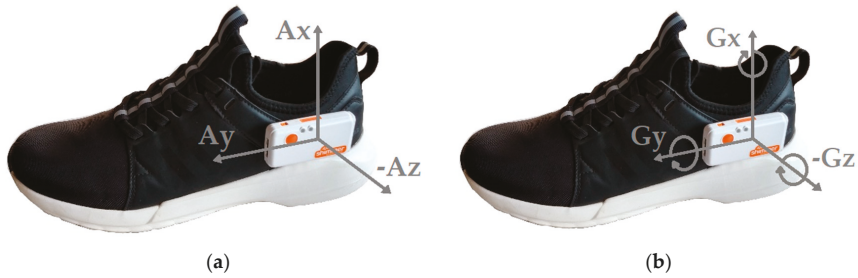
Figure 2. IMU sensor placement and axis alignment. (a) Accelerometer. (b) Gyroscope.
