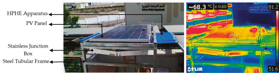
Figure 14. PV-HPHE apparatus isometric model (left) and captured infrared image (right) taken from the top surface assembled in the eco-house, Higher Colleges of Technology (HCT), Muscat, Oman.
