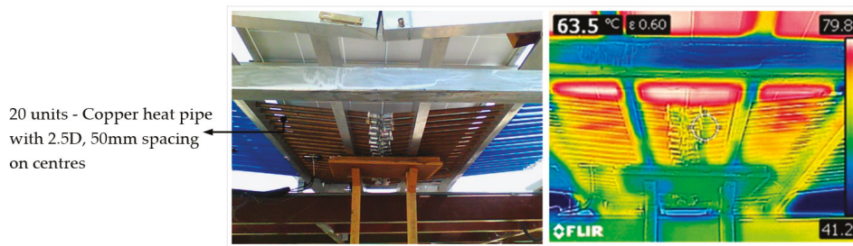
Figure 15. PV-HPHE apparatus isometric model (left) and captured infrared image (right) taken from the bottom surface.
